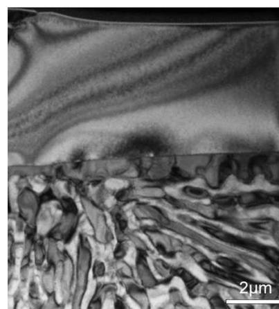
**Figure 3.** TEM bright field image of the microstructures. The TEM sample is milled perpendicular to one side of a hexagonal  $\text{Al}_2\text{O}_3$  grain and normal to the sample surface.
