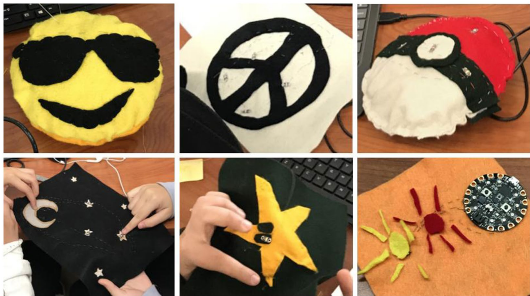
FIGURE 1 Examples of student teams' Debuglts (clockwise from upper left): Smiley face, peace sign, Pokémon ball, two suns, Mario star and 'Starry Night', which illustrate different aesthetic choices and configurations of circuit designs, LEDs and functionalities in code.
