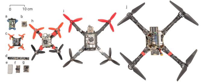
Fig. 1 Size comparison of various components used on quadrotors. (a) Snapdragon Flight, (b) PixFalcon, (c) 120 mm quadrotor platform with NanoPi Neo Core 2, (d) MYNT EYE stereo camera, (e) Google Coral USB accelerator, (f) Sipeed Maix Bit, (g) PX4Flow, (h) 210 mm quadrotor platform with Coral Dev board, (i) 360 mm quadrotor platform with Intel Up board, (j) 500 mm quadrotor platform with NVIDIA® Jetson™ TX2. Note that all components shown are to relative scale. All the images in this paper are best viewed in color on a computer screen at a zoom of 200%
