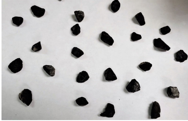
Figure 2: Some samples of the gravel pieces used in the experiment taken from gradation E.
