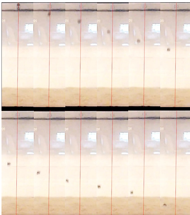
Figure 8: Series of 12 frame-by-frame images, showing a single piece of gravel falling through water. The vertical red lines correspond to the release location.
