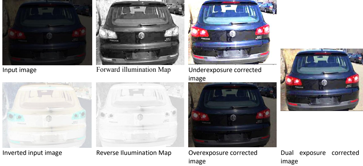
Figure 6: closer look at how the dual illumination module helps correct exposure in the input image.
