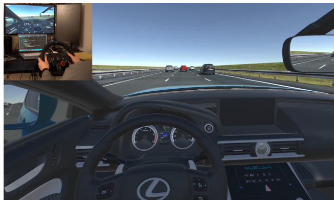
Fig. 4: Naturalistic driving in a car-following scenario with Unity game engine and Logitech racing wheel.
