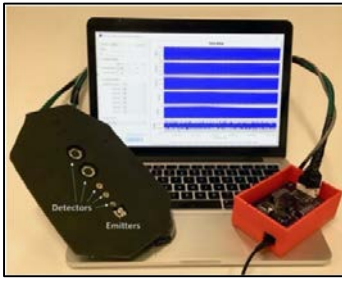
Figure 2. A picture of the prototyped Transabdominal Fetal Pulse Oximetry (TFO) system [13].
