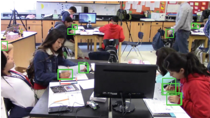
(e) Initial hand regions detected using Faster RCNN with significant hand movements.
