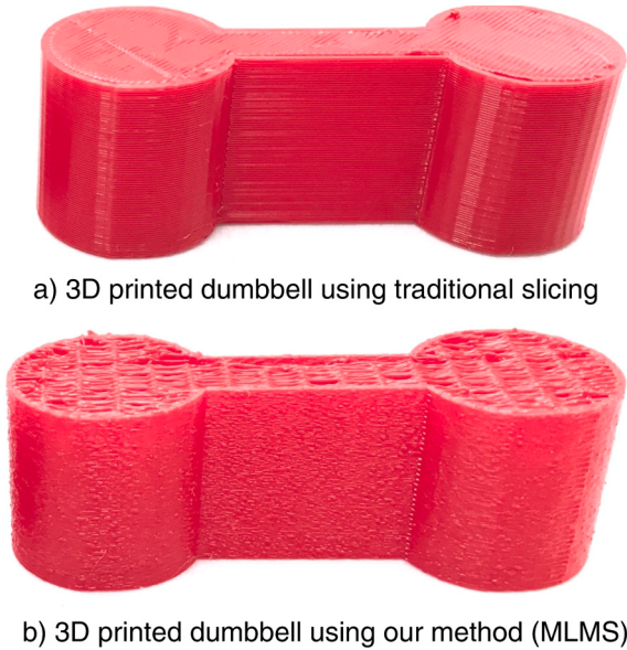
Fig. 19. 3D print comparison between the traditional slicing method and our direct 3D printing from multi-level voxels for a simple model.
