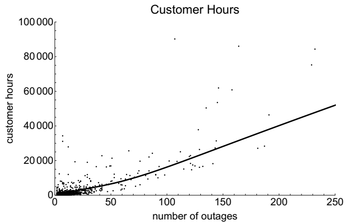
Fig. 11. Curve shows mean customer hours \bar{A} calculated from (28) versus number of outages. Dots show customer hours A of the events in the data.
