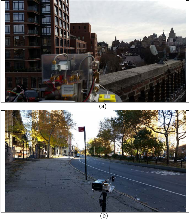
Fig. 1. (a) Spinning horn receiver overlooking West 11th Street in Manhattan from a roof edge 18 m above ground. (b) Omnidirectional transmitter placed in the middle of a sidewalk.
