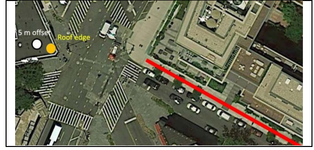
Fig. 2. Illustration of roof-edge (orange) and offset from roof edge (white), base antenna placement (on left). The same-street terminal is moved along the red line on right.
