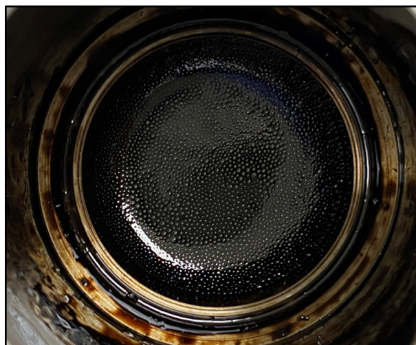
Fig. 12— N_2 dissolved in the crude oil being liberated at an injection pressure of 1,750 psi.
