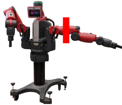
Fig. 2: Baxter, a compliant, two-armed, robot with 7-DoF arms used for this work. The red rectangle on the arm represents where the camera was mounted. Because ground truth was available from the encoders, no Vive trackers were used to estimate pose.
