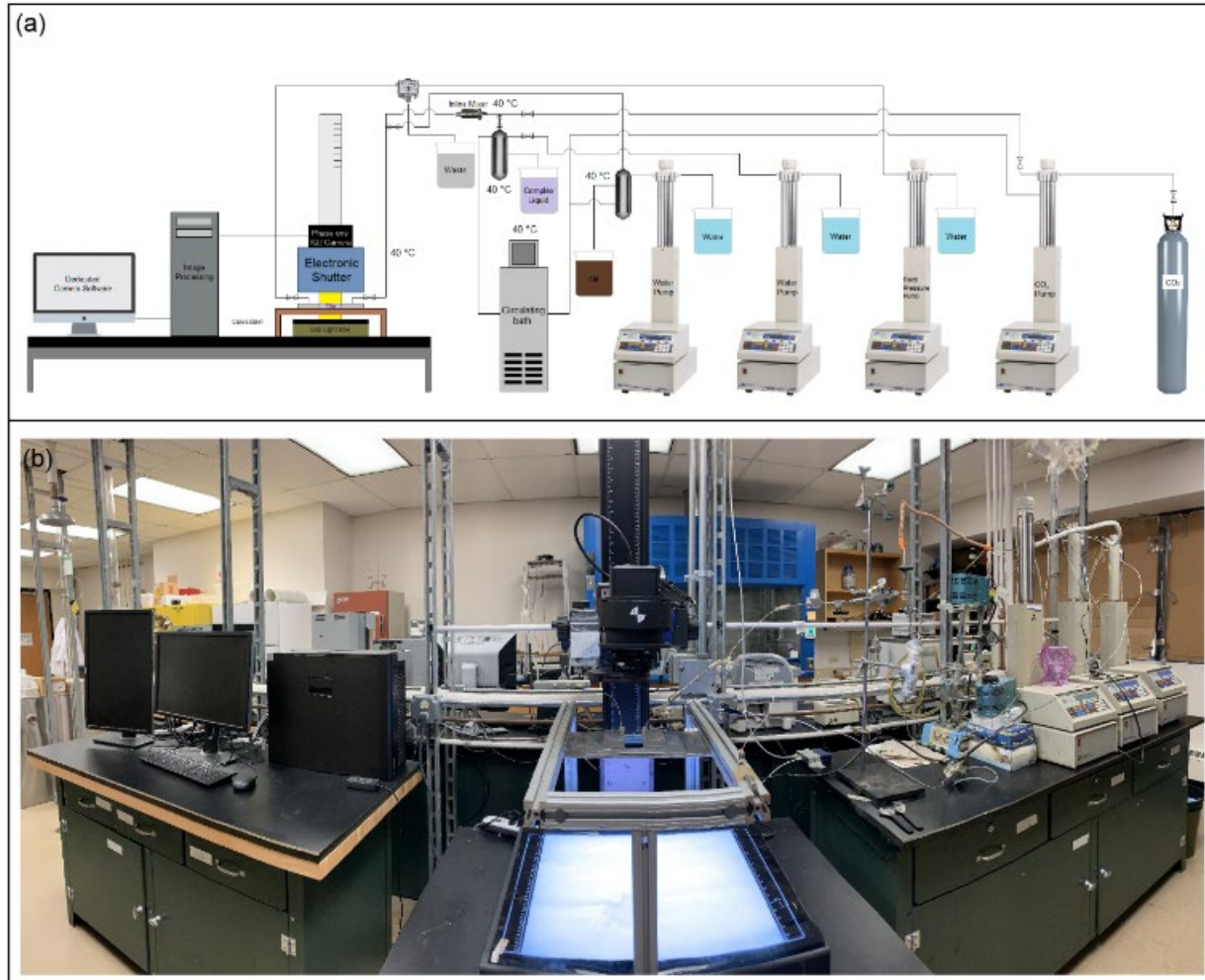
Figure 5. (a) schematic of high-pressure CO 2 foam injection and visualization of micromodel in laboratorial scale; the system is capable of scCO 2 foam generation as well as oil injection through the micromodels. Simultaneous visualization is performed using a high-resolution camera. (b) The photo of the actual setup in the lab, reprinted with permission from [31] JOVE 2020
