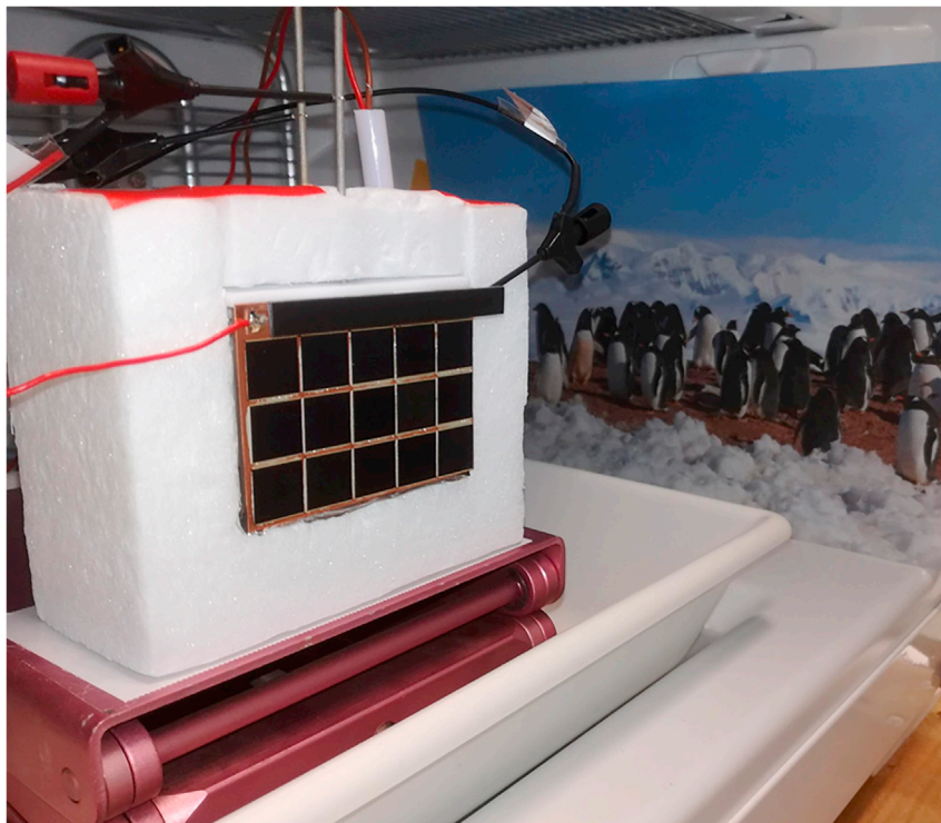
Figure 2. An image of the thermally integrated solar-water-splitting device studied by Kölbach, Rehfeld, and May
