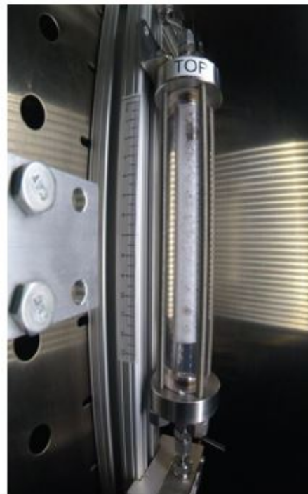
Figure 16. Static supercritical CO 2 foam at A) 70% B) 80% foam quality after 40 minutes
