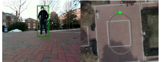
Fig. 3. Pedestrian detection (bold lines) and uncertainty (narrow lines) bounding boxes determined by the Gaussian Yolov3 detector (left). Top-down view of the track (right).
