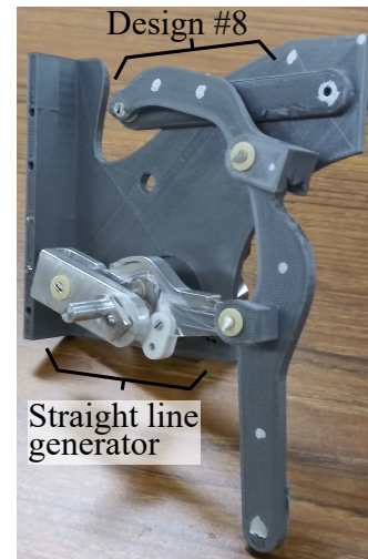
Fig. 9: A view of the partially assembled kinematic model.
