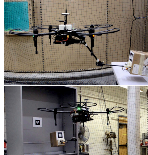
Fig. 1. Proposed aerial manipulation system picking (top) and placing (bottom) a package.
