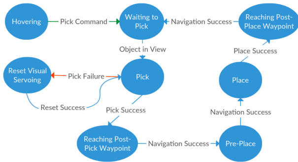
Fig. 6. Part of the state machine for picking and placing a package. The recovery actions are red and user actions are green. The user can also abort from any other state back to hovering if manual intervention is desired.
