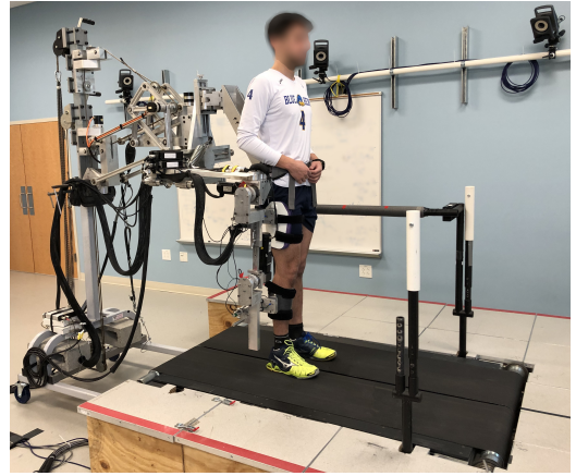
Fig. 1: Experimental setup consisting of a participant in the Active Leg EXoskeleton II (ALEX II) while on the instrumented split-belt treadmill.
