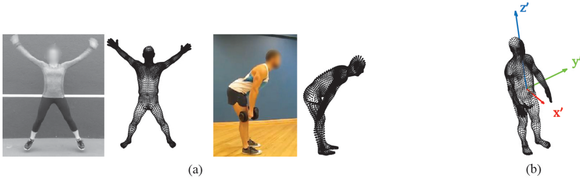
Fig. 2. (a) Sample reconstructed 3D human mesh from a snapshot of (left) a person doing jumping jacks and (right) a person doing stiff-leg deadlifts. (b) The Local Coordinate System (LCS), defined with respect to the human body.
