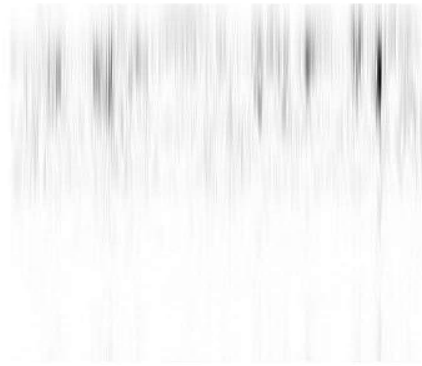
Figure 6: The F-scan from Figures 5a and 5b laid flat on a 2-D plane in the style of a B-scan
