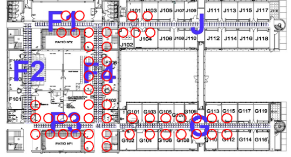
Fig. 2. Testbed used for our studies. All 50 devices are deployed on the same floor in an office building. One device serves as the border router (Root) and the rest are end devices.
