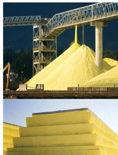
Figure 2. Examples of megaton above ground sulfur storage sites resulting from refining of petroleum via the Claus process. Adapted with permission from ref 31. Copyright 2016 Elsevier.
