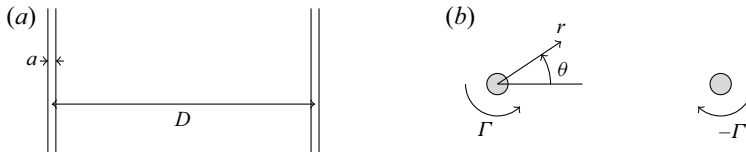
Figure 1. (a) Side view of two parallel vortex tubes and (b) a cross-section view of the counter-rotating vortices. The shaded areas are occupied by fluid of density \rho_2 , whereas the ambient density is \rho_1 .
