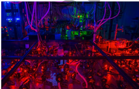
Figure 1. (left) Atom-based experiments in quantum science like this lithium quantum gas apparatus typically utilize benchtop equipment and free-space optics which dominate the cost and complexity and restrict scalability. (right) Properties of some atomic transitions of general interest.
