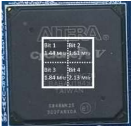
Fig. 14 Location and the frequencies of modules that create the 4 bits.
