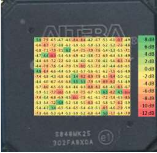
Fig. 17 Relative strength of bit 1 compared to other bits.
