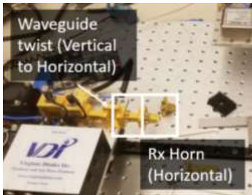
Fig. 8 The measurement setup using polarization filtering.
