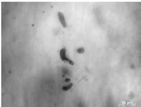
FIG. 4. Optical image of inclusions in sample C3. Image obtained with a Zeiss Axio Observer A1 microscope.
