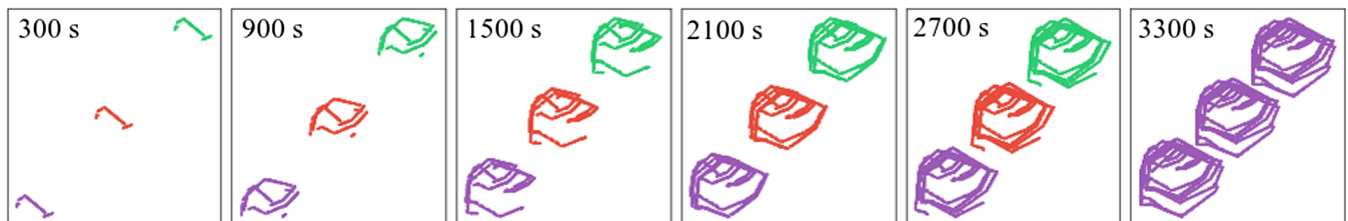
Fig. 15 Hierarchical clustering results for three fires growing toward each other. Snapshots from left to right are at progressive simulation times with colors denoting group membership.
