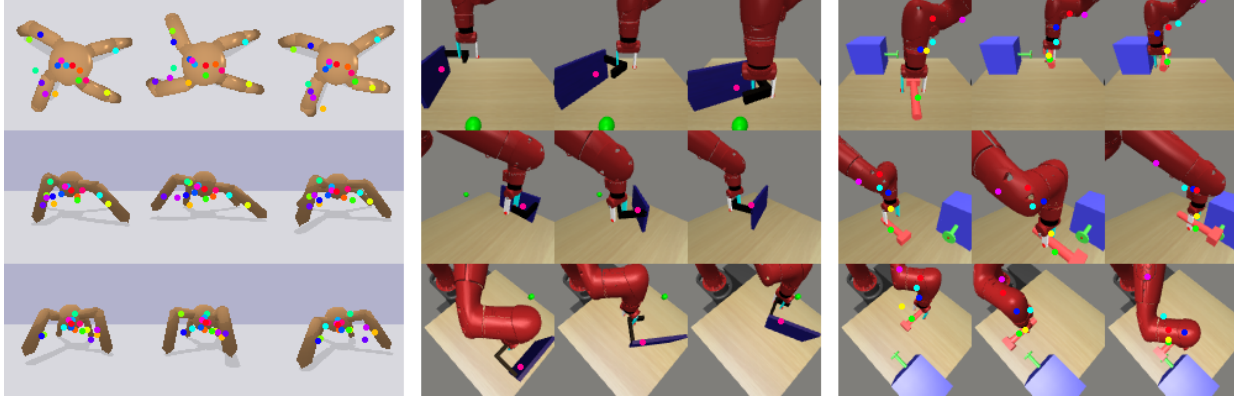
Figure 7. Visualization of the learned keypoints on colorless ant (left), metaworld close door (middle), metaworld hammer (right) environments. For the two metaworld environments, we filter keypoints with a threshold on learned keypoint attention. In colorless ant, the keypoints consistently track the limbs. In door the pink point with highest confidence tracks the movement of the door consistently. In hammer, the green point tracks hammer, while other points tracks the end-effector and sections of the arm respectively.
