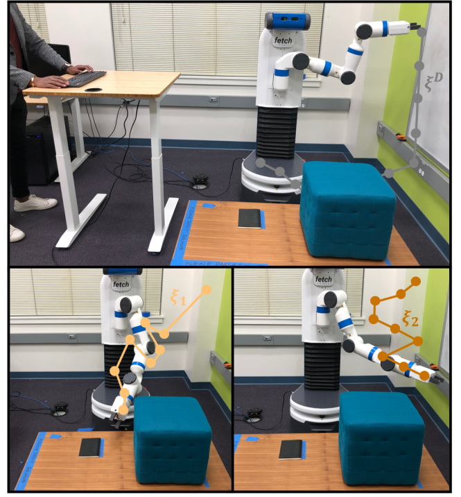
Figure 2. Example of a demonstration (top) and preference query (bottom). During the demonstration the robot is passive , and the human teleoperates the robot to produce trajectory \xi^D from scratch. By contrast, the preference query is active : the robot chooses two trajectories \xi_1 and \xi_2 to show to the human, and the human answers by selecting their preferred option.
