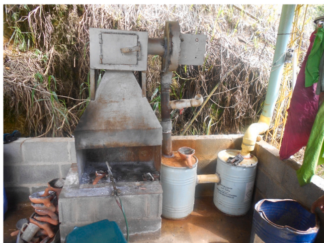
Fig. 2. Example of a fume hood system attached to a series of water barrels meant to capture mercury vapor before releasing gases into the atmosphere. Materials are burned in clay bowls under the mouth of the fume hood. A fan draws the vapors through the mouth and down through a series of water barrels. The remaining vapors are released (not shown).
