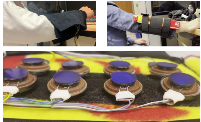
Fig. 1. System Setup: (top-left) person with sensor sleeve, (top-right) person with voice coil sleeve, (bottom) voice coils inside the actuation sleeve.
