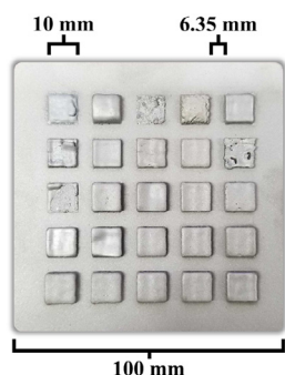
Fig. 2. Photograph of the as-built Cr-Fe-Mn-Ni array printed on a 316-stainless-steel build plate after media blasting to remove adhered powders. Prior to any machining, sample heights and surface finish as printed vary as a function of composition.
