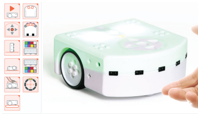
Figure 2: An example of coding blocks in the Thymio bot's VPL (left) next to an image of the Thymio bot (right).
