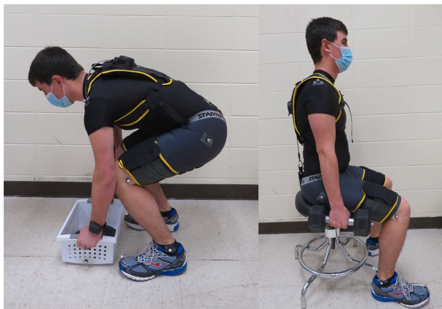
Fig. 2. A participant performing two tasks while wearing the exosuit and sensors: lifting a box from the floor (left) and standing up from a stool while holding dumbbells (right). Optical tracking markers are visible on the body and lifted objects, and the heart rate bracelet is visible on the left wrist. Electromyography sensors are not visible from this angle.
