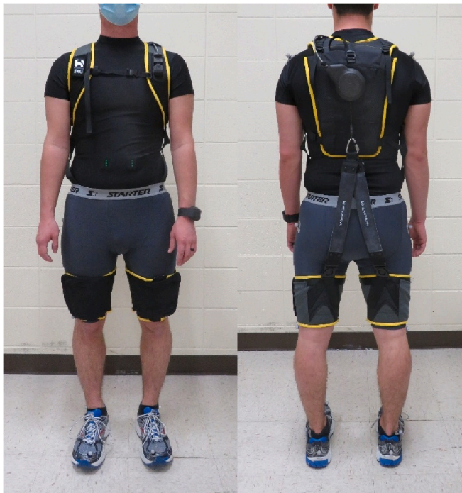
Fig. 1. A participant wearing the Apex (HeroWear, Nashville, USA), front and back views. The exosuit consists of an upper-body part similar to a backpack, two thigh sleeves, and two elastic bands on the back that connect the upper-body part to the thigh sleeves. The participant is also wearing the sensors used in the study (e.g., wireless electromyography sensors under shirt, optical tracking markers on shoulders, heart rate bracelet).
