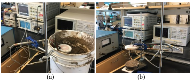
Fig. 8. Experimental setup for wireless power transfer: (a) through 15 cm loamy soil and (b) across 15 cm air.
