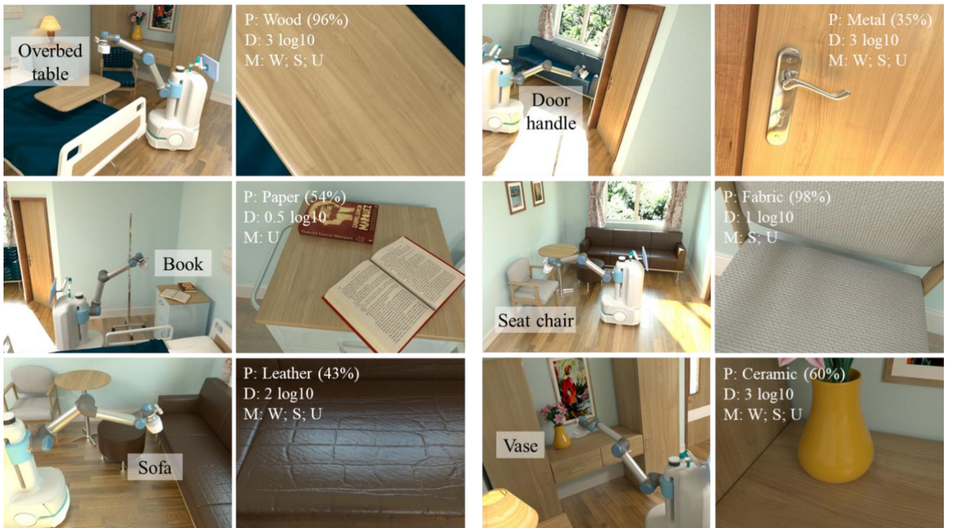
FIGURE 12. Example results of material classification on images captured by the robot. P: predicted material (confidence value in parentheses); D: disinfection dosage; M: disinfection mode; W: wipe; S: spray; U: UVC light
