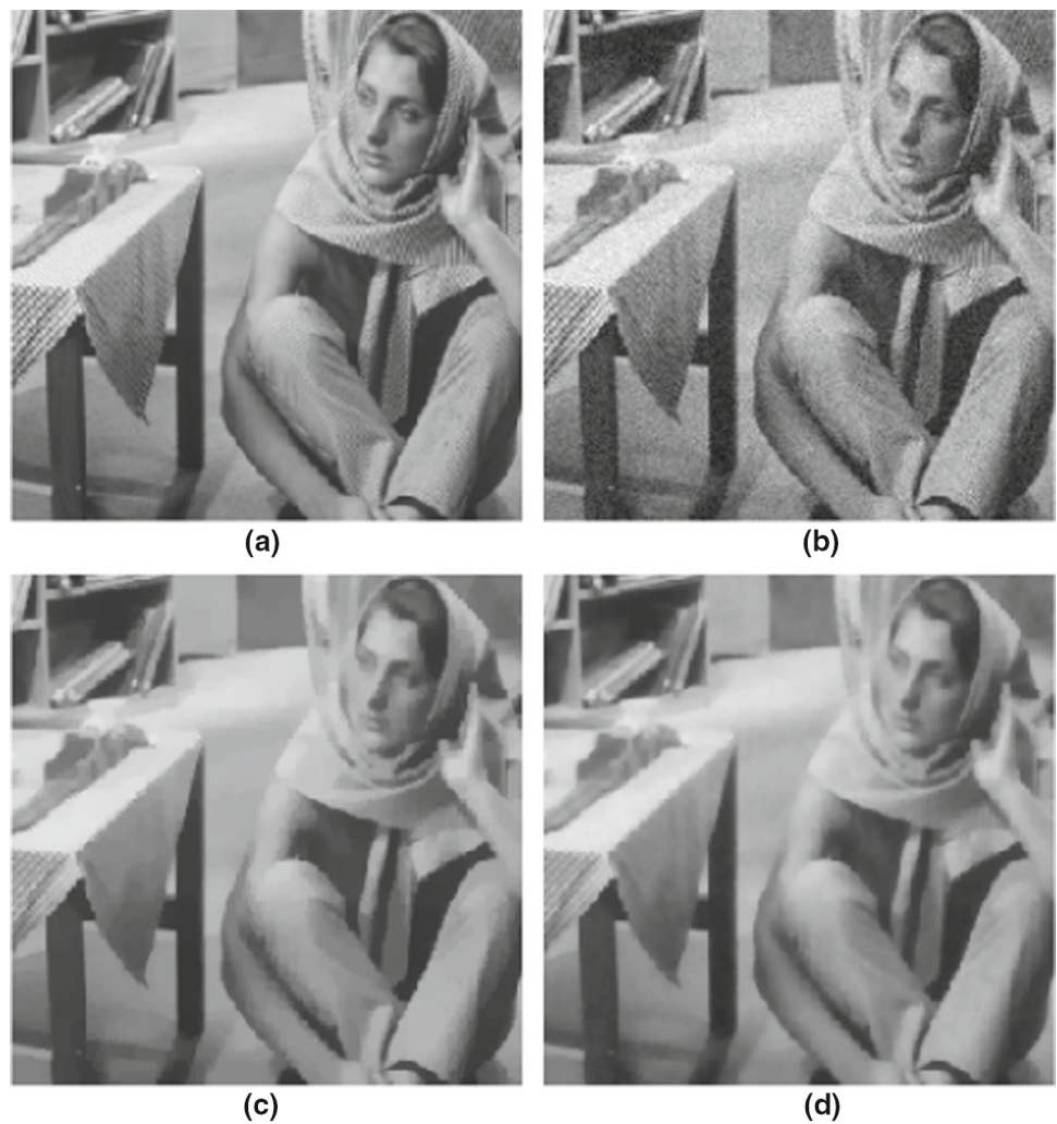
Fig. 1 The anisotropic ROF model endowed with 4-nearest neighbors is applied to the test image “Barbara”. The original image is shown in (a). The image is corrupted by Gaussian noise (zero mean with standard deviation \sigma = 10 ) and is shown in (b). The corresponding minimizer u_{MAP}(x, t) given by (4) and posterior mean estimate u_{PM}(x, t, \epsilon) given by (6) with parameters t = 16 and \epsilon = 6.25 is illustrated in (c) and (d), respectively
