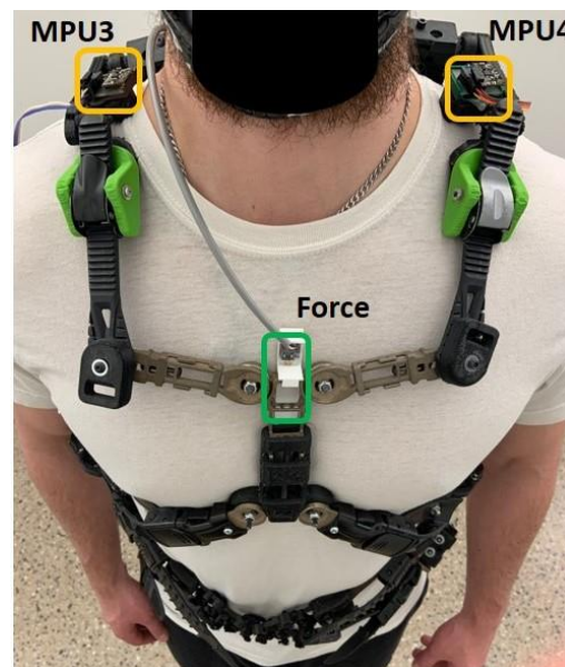
Figure 2. The trunk exoskeleton worn by a person, front view. Motion processing units (MPUs) and force sensor are highlighted.
