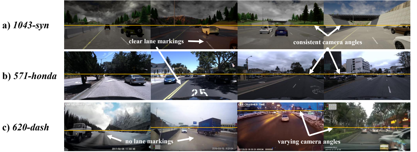
Fig. 4: Examples of driving scenes from our a) synthetic datasets, b) typical real-world dataset, and c) complex real-world dataset. In a), all driving scenes occur on highways with the same camera position and clearly defined road markings; lighting and weather are dynamically simulated in CARLA. In b) driving scenes occur on multiple types of clearly marked roads but lighting, camera angle, and weather are consistent across scenes. c) contains a much broader range of camera angles as well as more diverse weather and lighting conditions, including rain, snow, and night-time driving; it also contains a large number of clips on unpaved or unmarked roadways, as shown.
