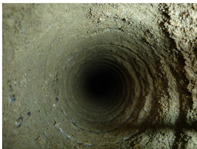
Figure 2. Photo of borehole after completion with gasoline-powered auger. Ice is visible along the walls where the soil was abraded, demonstrating the limited thermal effects of drilling.
