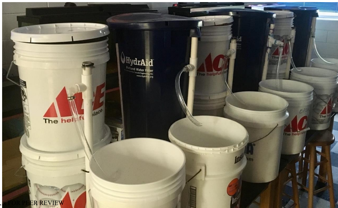
Figure 3. Two bucket BSFs and HydrAID commercial BSFs in the high school laboratory.
