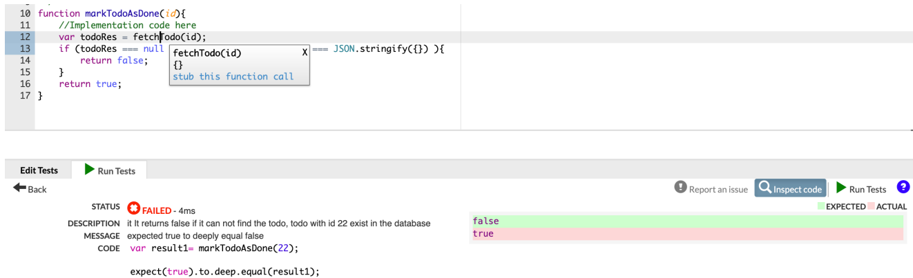
Figure 6: Workers can debug failed tests by using the Inspect code feature to view the value of any expression. In cases where a function that is called from the function has not yet been implemented, any tests exercising this functionality will fail. To enable the worker to still test their contribution, a worker may create a stub for any function call.
