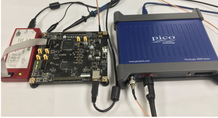
Fig. 6. The evaluation setup for the side-channel experiments with the Picoscope 3206D oscilloscope.
