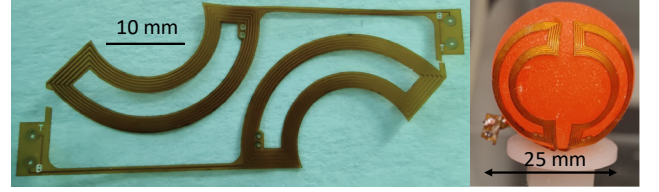
Fig. 2. Optical images of a pair fabricated scleral coil (left) and coil mounted on polymeric sphere (right).
