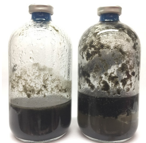
Figure 3. Municipal wastewater collected from the Theresa Street Water Resource Recovery Facility in Lincoln, Nebraska. (Left) Organic solids before anaerobic digestion. (Right) Organic solids after anaerobic digestion.
