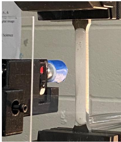
Fig. 5 Sample testing with MTS machine and PS system
