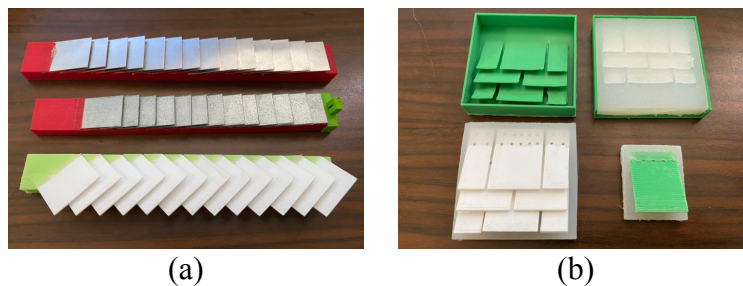
Figure 1. (a) Fabricated 1D scale-covered prototypes using glue the stiff scales into prefabricated grooves of deformable substrate. (b) Fabricated 2D scale-covered prototypes using female mold to arrange scales in a 2D overlapped arrangement.
