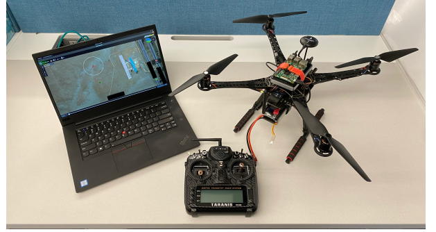
Figure 4: Hardware setup showcasing the Holybro S500 drone, the radio controller, and the ground control station.
